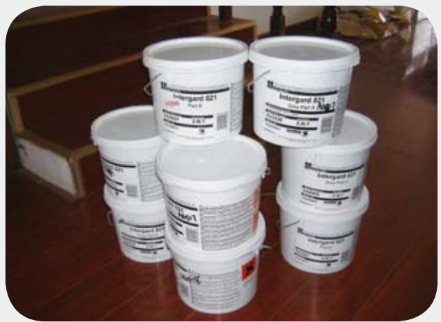
Epoxy filler for ICCP Di-electric shield
